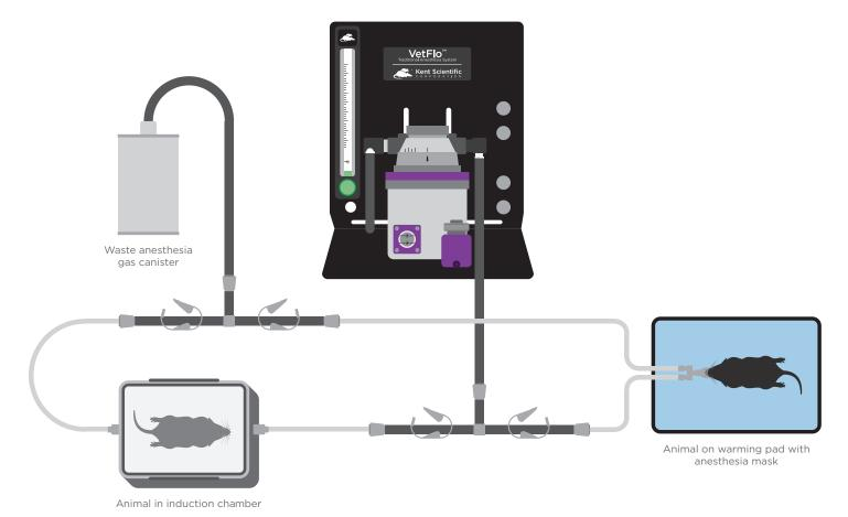
Perfect for laboratory and veterinary anesthesia delivery, the VetFlo vaporizer is completely self contained and portable. The multi-channel base is designed for multiple stations that are individually controlled. You can work with up to six stations, operating off of one vaporizer. With an easy-to-follow chart,
