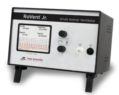
RoVent and RoVent Jr. small animal automated ventilator are ideal for mice, rats and small animals up to 1,250 grams. Both are fully automated — simply enter the animal's weight and press run.
